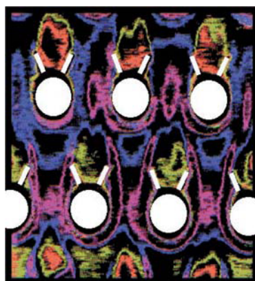
Fig. 6. Colour-scale representation of Nusselt number for staggered cylinders. Re = 1600 (Nusselt number: red - 5.27; green - 7.99; blue - 15.38; violet - 19.17).
